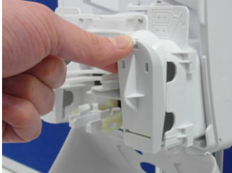
Depress retaining tab to open battery door.
