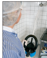
9. The distance from the injectors nozzle-opening to the cleaning surface has to be minimum 50 cm.
