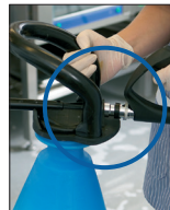
6. The water gun (item no. 93209 or 93219) is connected to the nipple on the injector.
