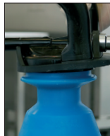
5. Screw the injector tight on the container.
