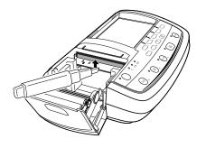
To protect the thermal head from abrasion or damage and assure optimum performance and long service life, clean the surface of the head with the provided thermal head cleaning pen after every 10 sets of recording paper.
