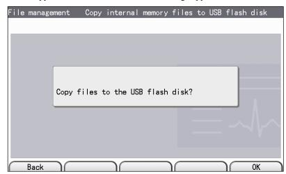
Press the [OK] function key to copy the files. A "Copying. Do not turn power off" message appears.
